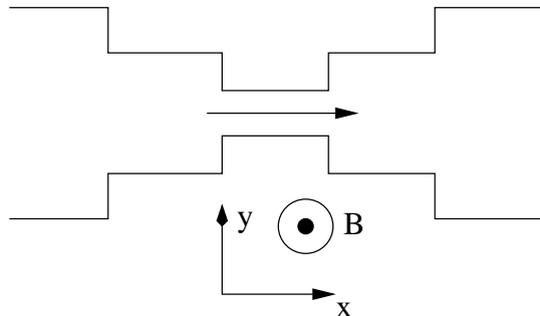
Figure 1: Schematic representation of a QPC, produced by lateral confinement of a 2D electronic gas.
