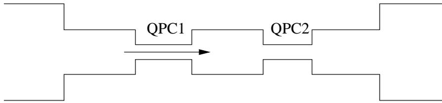
Figure 2: Schematic representation of a system of two identical QPCs in series.
