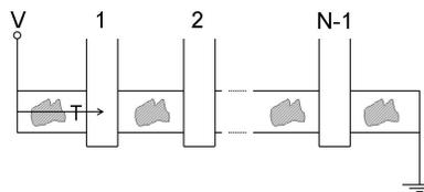
**Figure 2.** Schematic representation of a physical system consisting of  $N$  scattering regions with phase coherence, connected by voltage terminals.
