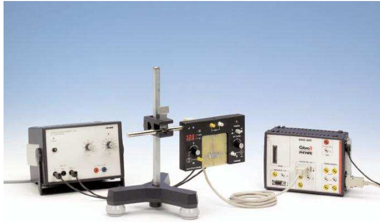
Fig. 4.3. Experimental setup for the determination of the band-gap of germanium.
