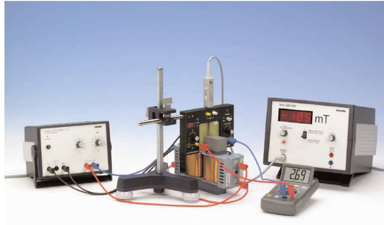
Fig. 6.2. Experimental setup for temperature dependent Hall effect measurements.
